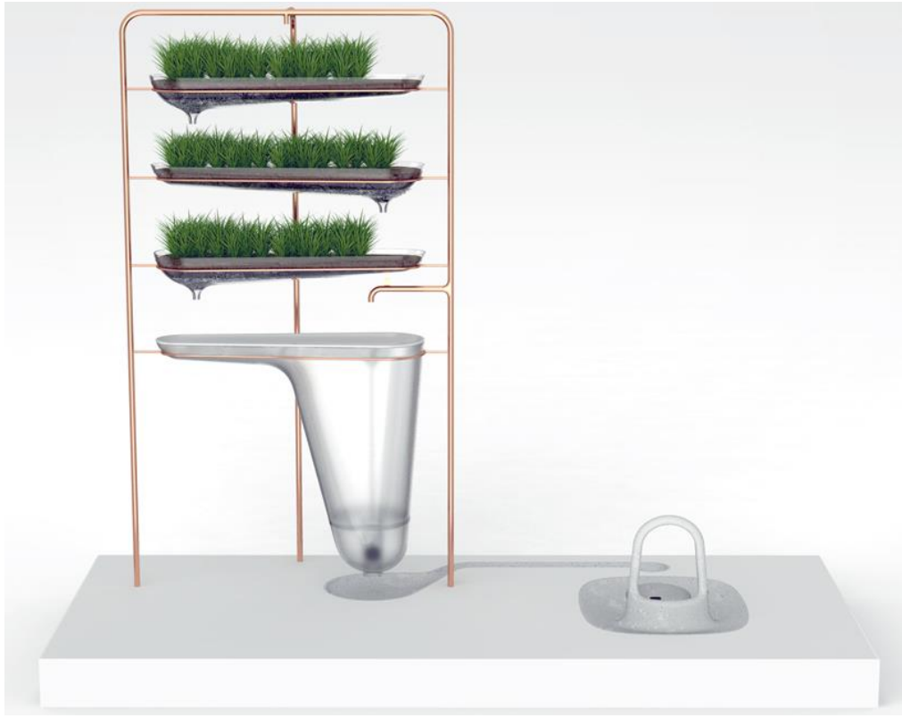
Figure ix: The squat-toilet station of the Microbial Home, incorporating a methane bio-digester to generate energy from excrement; urine is sent through a system incorporating plants, which it fertilises while it is filtered.*
